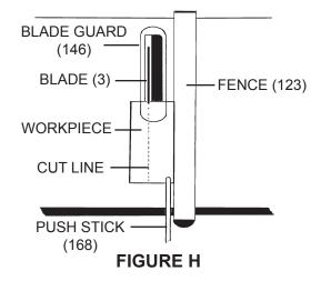
5. At the start of the cut, the left hand holds the workpiece firmly on the Work Table (86) and against the Fence (123), The right hand, with the aid of the Push Stick (168), pushes the workpiece toward the turning Saw Blade (3). Always keep both hands a safe distance from the spinning Blade (3). See **Figure H**, above.
